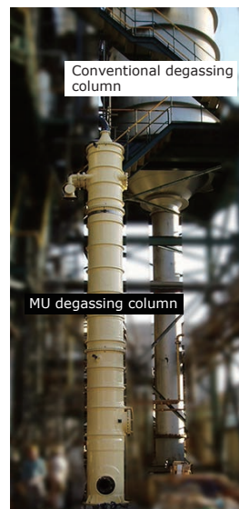
Photo 1 Comparison between conventional and MU degassing tower
