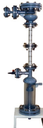
Gas-liquid contact part of MU Reactor system ( \phi 34 \times 600H )
