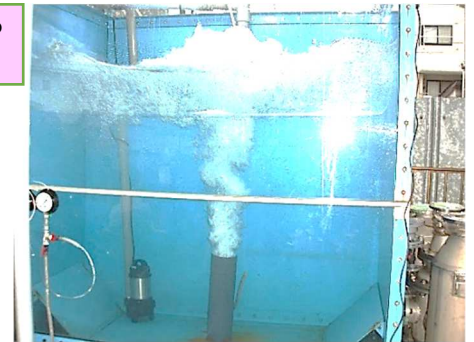
Photo-3 [Reference] Aeration agitation status of the Mu-Aerator
